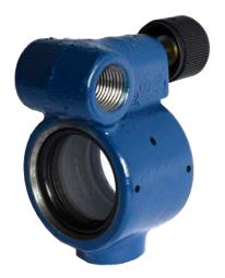
The Model 4B Gravity Sight Feed Oiler offers a clear oil flow view with fine tune-control. The Model 4B allows oil flow by gravity to a lubrication point. The double-window design permits observation of the oil stream from either side. This oiler provides trouble-free service with little or no maintenance required. Its compact design ensures easy installation in confined spaces, and the corrosion-resistant materials guarantee durability even in harsh environments.
