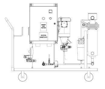
The Turbo-TOC<sup>®</sup> KLP Series provides the same fluid cleanliness performance as the KL line in a compact, mobile platform designed for systems up to 1,800 gallons. Ideal for service teams or facilities with multiple smaller reservoirs, KLP units deliver ISO-compliant particulate and water removal with field flexibility, making them a strategic solution for planned maintenance, commissioning, or rotating equipment support.
