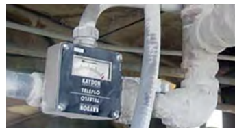
Close-up view of Model 816BC TELEFLO® Flow Switch mounted on rock crusher lube oil (ISO 150) circuit for protection against loss of oil flow in quarry application.
