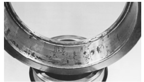
Bearing failure from excess water
