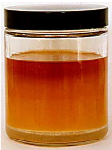
Figure 1 Dissolved, emulsified and free water in oil, with a biological contamination at the water interface.
