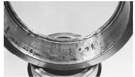
Bearing failure from excess water
