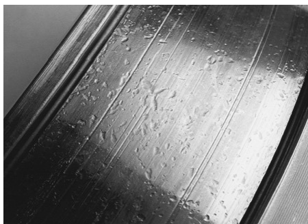
Fatigue wear results induced by pressure and accelerated by water in oil.
