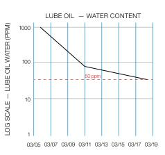
The KL30S2 Turbo-TOC® system was installed when water content was almost 1000 ppm. After a few days of use the system reduced water content to less than 100 ppm.
